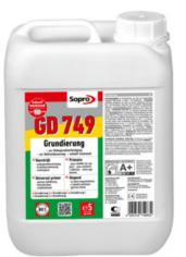
Quick-drying, highly concentrated, solvent-free, synthetic resin primer for high- and variable-suction substrates. For pretreatment of cement screeds, calcium sulphate screeds, board subfloors, gypsum plasterboard and gypsum fibreboard, lime/cement render and gypsum plasterwork. For subsequent application of mineral adhesives, surface fillers and waterproof membranes. Dilutable with water to suit application. Apply to gypsum-bound substrates in undiluted form.
