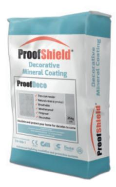
**ProofDeco Mineral Render** is a polymer modified, mineral render top coat with the benefit of hybrid silicone additives for enhanced weather protection. It is suitable for use as a breathable top coat over **ProofTherm Insulating Render**, to finish off ETICS systems and as a general purpose decorative render at thicknesses up to 7mm.
