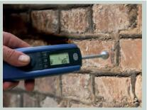
APPLICATION It is of importance how the unit is held while measuring: The BL Compact B 2 unit should be held at the rear part of the unit and applied to the material to be measured in a 90° angle.
