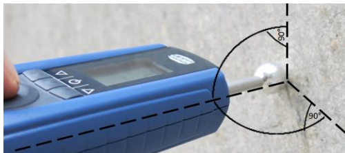
Figure 4-3 Measuring as vertically as possible to the measurement are
